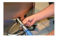
**Connecting to the gun:** Plug the male connector on the gun into the female socket on the blast hose, again, by inserting the plug and twisting clockwise.
