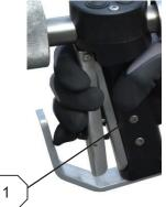
The blast gun has for safety been equipped with a safety pin (1) at the trigger. In order to activate blasting the lever most be pushed down, which in turn allows the trigger to be pressed.
