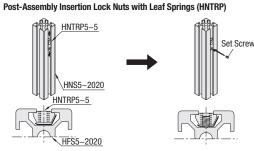
Welded Leaf Springs maintains position (even in vertical extrusions), leading to easy locating.
