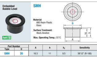
**Bubble Levels** - This bubble level is for mounting on a surface that has already been checked to ensure it is level, and it provides a simple level check. Fit it so that the bubble is stationary within the red circle. (A shim or adjustment mechanism may be required depending on the surface accuracy.)
