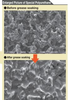
Special polyurethane has interconnected micropores and is excellent in waterholding capacity. Enables to impregnate much grease.
