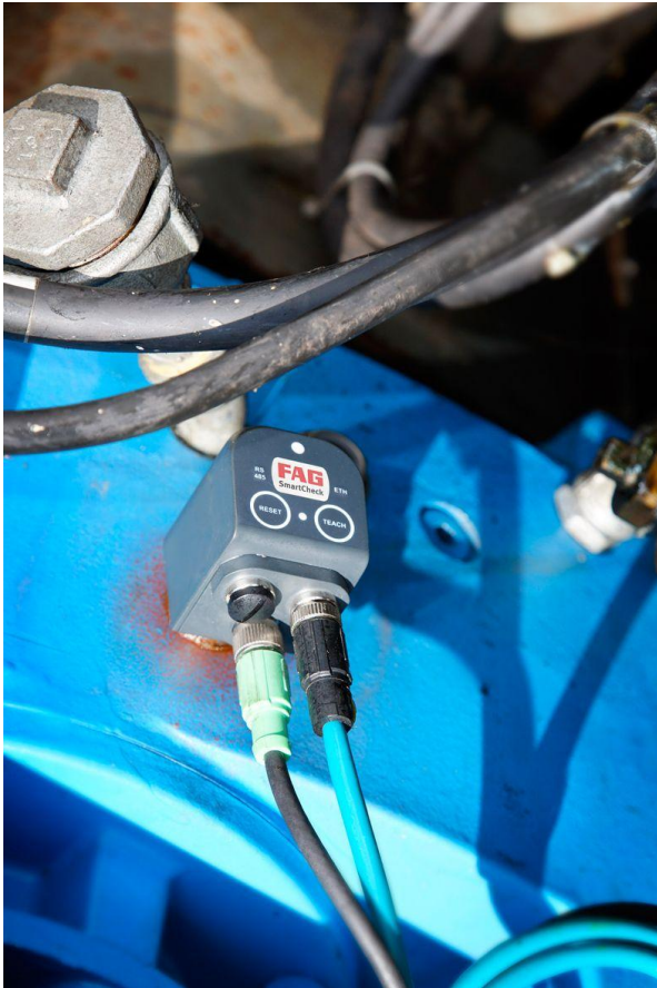
FAG SmartCheck Unit Installed At Rotenburg an der Fulda Plant
