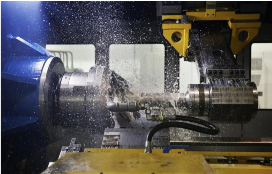
Advanced Manufacturing: WF Flow Former For High Precision Rotationally Symmetric Products. Source: University of Strathclyde, UK
